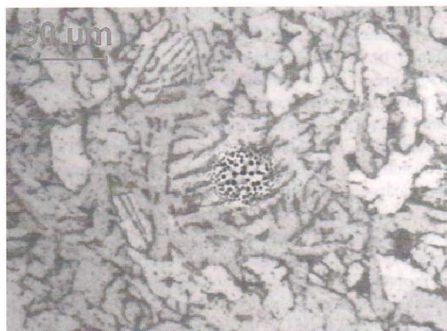
Fig. 9: Optical micrograph of KRD-5914 showing the predominance of ferrite
