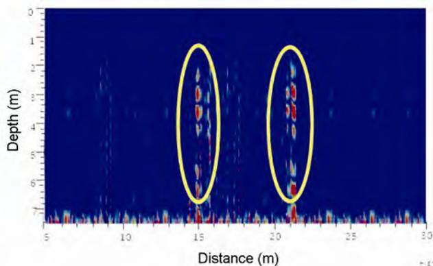
**Figure 7.** Improved GPR profile along NS direction of area A1 using time-frequency analysis.
