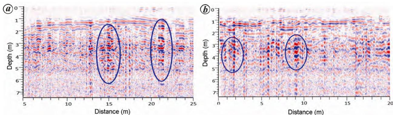
Figure 3. Select GPR profiles showing marked signatures across linear features along (a) NS direction in area A1 and (b) EW direction in area A5.
