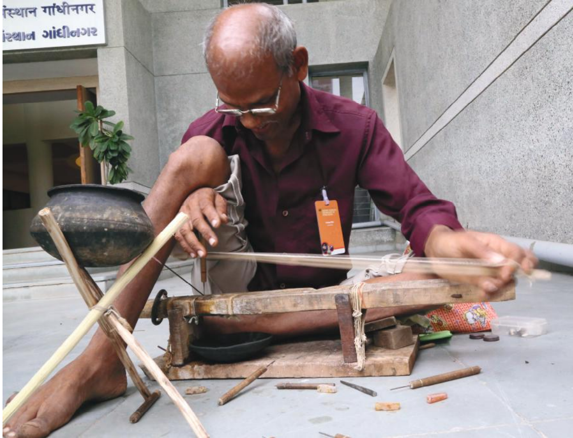
Figure 9: Craftsman Pratap Bhai demonstrating drilling
